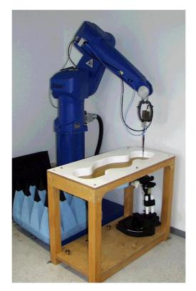
Fig. 7: The measurement setup with a phantom containing tissue simulating liquid and a device under test.
